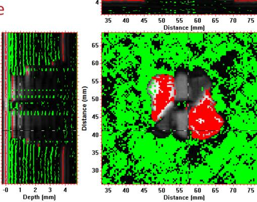
Green: Resin layer. Red: front, back or delamination. Note: multiple reflections are not colour coded
