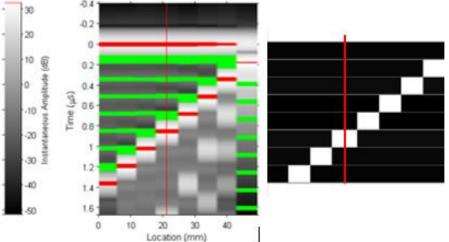
Simulated data for delaminations in an 8-ply composite Green: Resin layer. Red: front, back or delamination. **Note: multiple reflections are not colour coded**
